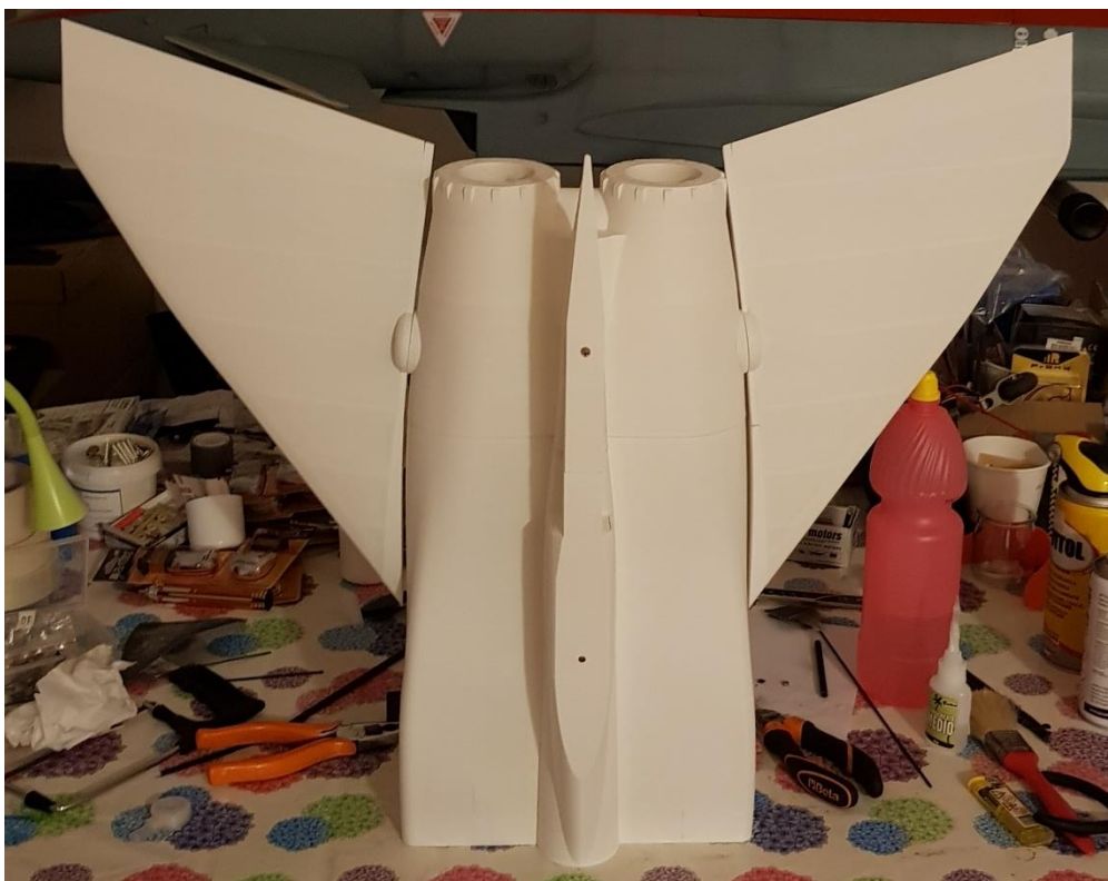
Glue the two fuselage sections with cyano acrylate glue
