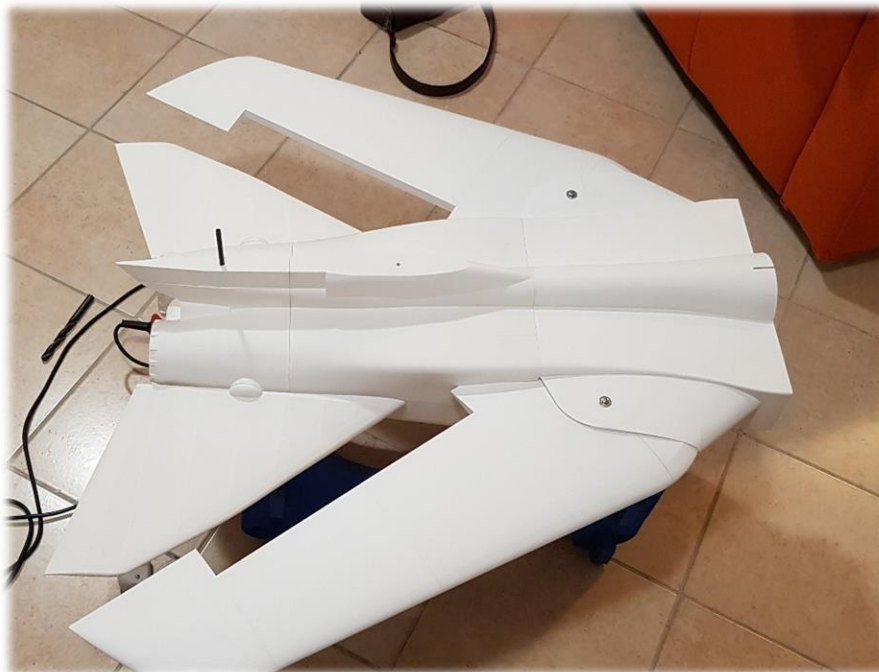
At this point glue the section with cyano acrylate and connect the wings
