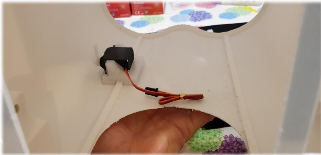
Detail of the installation of servo inside the fuselage
